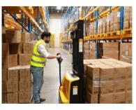
Easily maneuvered with the handle in the vertical position by pressing the turtle-speed button.
